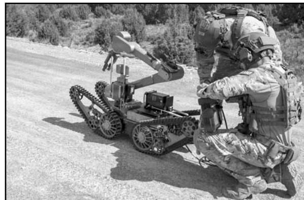
BOMB ROBOT Explosive ordnance specialists show a demonstration of a 'telerob,' a robot designed to help personnel stay out of harm's way while disarming explosives, in support of Exercise Wolverine, April 26, 2026. Utah National Guard photo by Senior Airman Kyle Blackham
