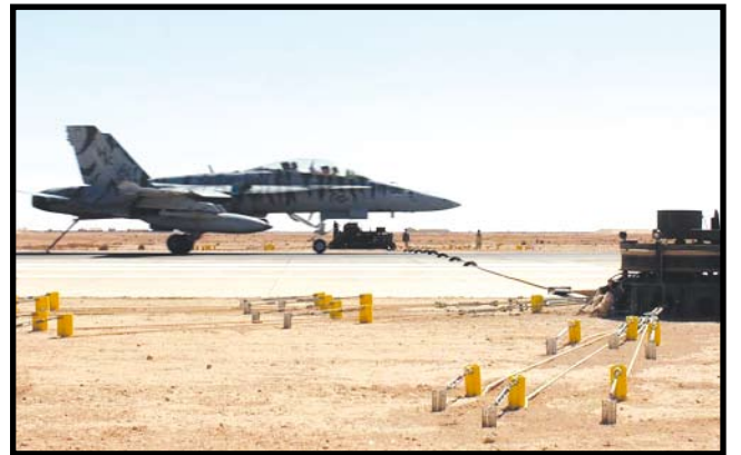
Arresting gears being utilized on land-based landing. Photo courtesy of Naval Air Systems Command
