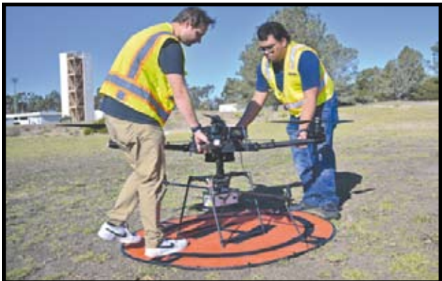
VENTURA TESTS Mechanical engineers with NAVFAC Engineering and Expeditionary Warfare Center Kaulin Hall and Kevin Vargas move a multi-rotor drone into place for test flights at Naval Base Ventura County Jan. 2, 2025. The drone is used to make high-resolution ortho-mosaic maps and can be used to support planning operations of expeditionary construction. U.S. Navy photo by Lisa Ferdinando
