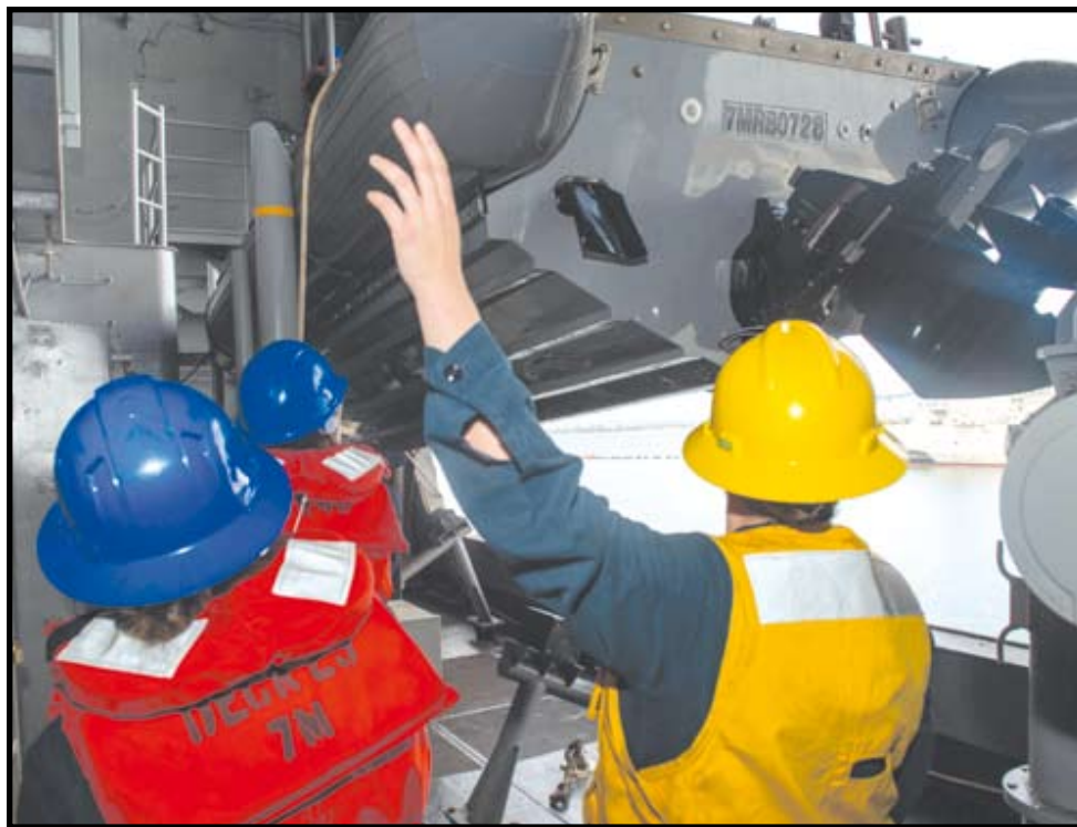
Boatswain's Mate 2nd Class Jocelyn Newsom, right, assigned USS Essex, directs the operator for the slewing arm davit to lower a 7m rigid-hull inflatable boat (RHIB) during small boat operations aboard Essex. U.S. Navy photo by MCSA Aaron J. Rolle
